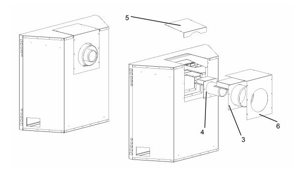
The appliance is easily converted from top vent to rear vent.
